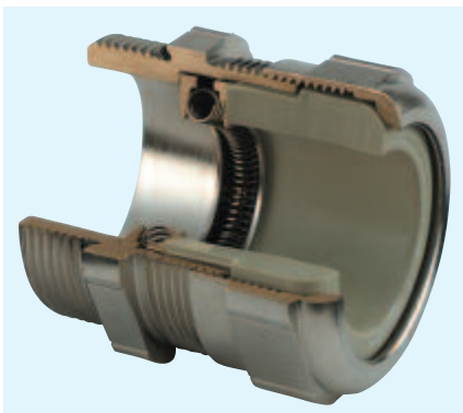
Fig. 2 The screen is bonded on its entire circumference (360°). The upshot is a low-resistant live connection between the screen, gland and housing.
