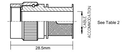
REWORKABLE BAND CLAMP & BRAID FOR INDIVIDUAL AND OVERALL SCREEN TERMINATION
